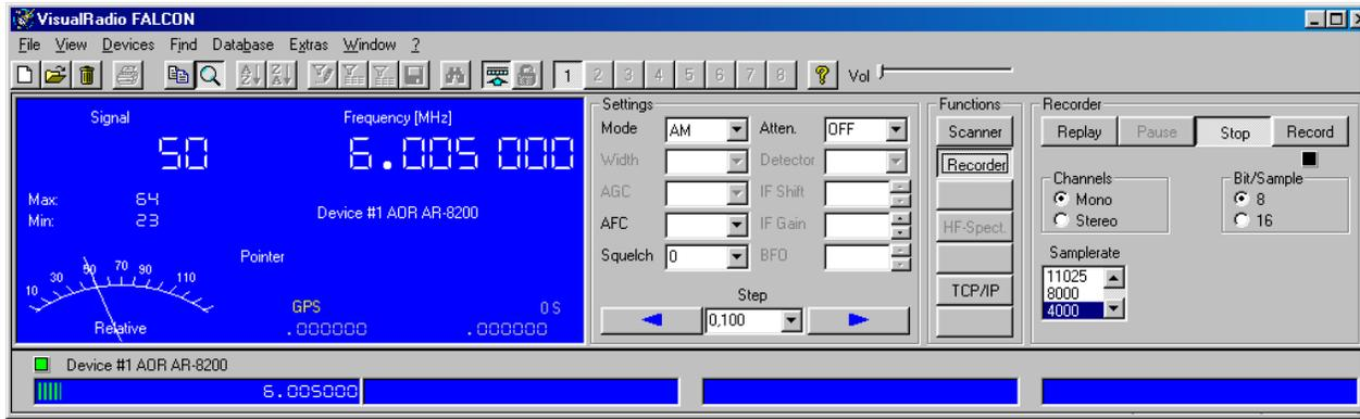
1. Signal displays for main and sub receivers, in case of a direction finder there are also the indicators for 'Bearing' and 'Quality'
