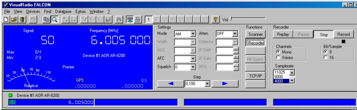
Displays various parameters of the tuned station.
