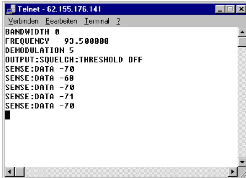
Here you see that VisualRadio Server has sent relevant parameters to the client (Telnet), when the link has been established. These parameters are the bandwidth, frequency and so on. After this initialization, the signal level is continuously transmitted.
