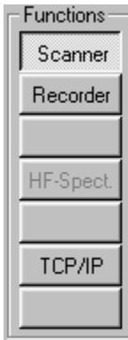
If the Recorder Panel, HF-Spectrum Panel or the TCP/IP Panel was previously displayed it will be replaced by the Scanner Panel
