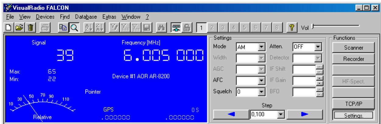
and the additional function panels like 'Scanner', 'Recorder' are displayed in place of the original 'Settings' panel, i.e. panels are 'stacked'
